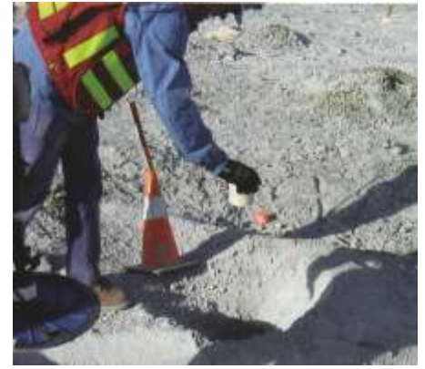
Placing a BMM in a blast hole to monitor ore movement during blasting
